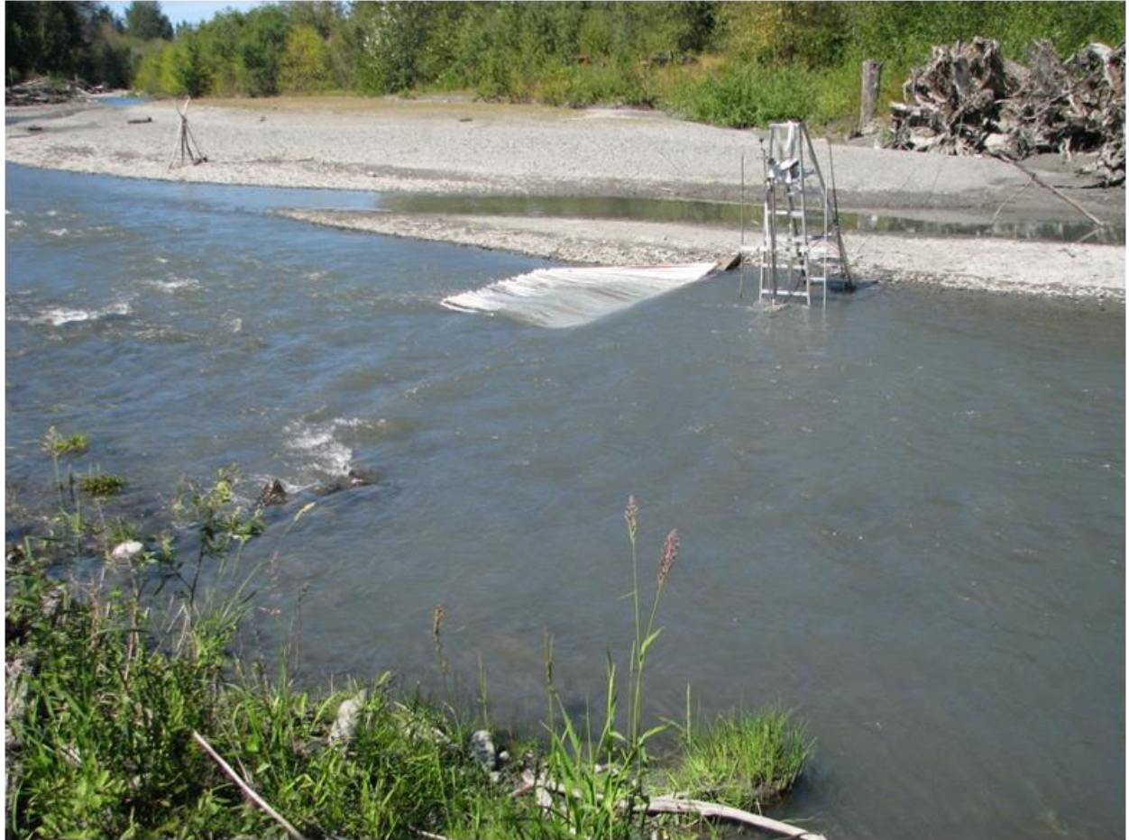
Figure 4. East Channel SONAR site. The SONAR is attached to the pole mount which is in turn attached to the ladder. The PVC picket weir immediately downstream from the ladder directs fish away from the bank so they pass at least 3 m from the SONAR head.
